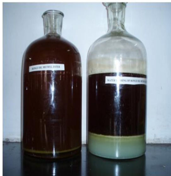
Figure 6: Washing and moisture removal from JOME
