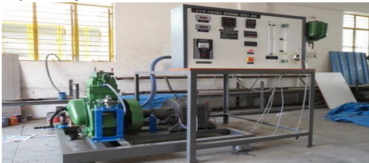
Figure 1: Four stroke diesel engine setup in Lab
